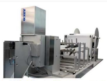
AZCO Corp. (Fairfield, NJ) has designed and manufactured a custom cut to length system with a material flow package, pleating station and heat set station. The application required unwinding gauze from a roll, folding it into pleats, pressing it and then cutting it to length. Specifically:
